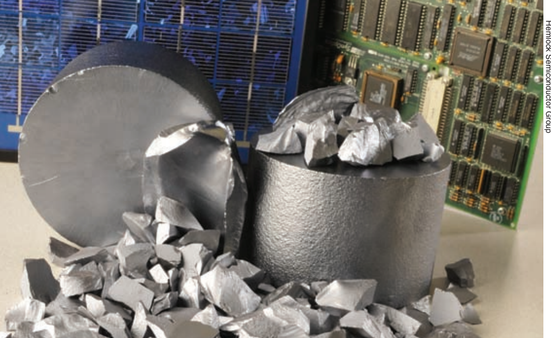
Hemlock Semiconductor Group bought a site in Clarksville, Tenn., to make polysilicon for the solar industry. The investment will amount to $1.2 billion, creating 500 full-time jobs and more than 800 construction jobs. The gray material (above) is polysilicon, or polycrystalline silicon. In solar applications, it is the cornerstone material used to produce solar cells that harvest renewable energy from light rays. The material is also used in the production of semiconductor devices.
